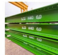
<鋼製山留主材H-40>
